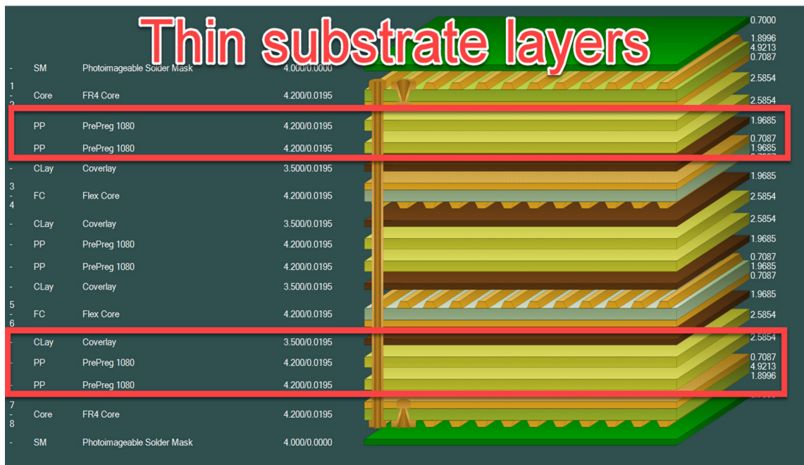
Real thicknesses of substrate layers
