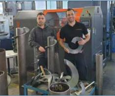
With SOLIDWORKS simulation capabilities, RoboHelix engineers were able to dial in the force required, and in what direction it should be applied, to achieve the controlled deformation through which the company's robotic flight-forming machine stretches a metal disc to form a helical flight.
