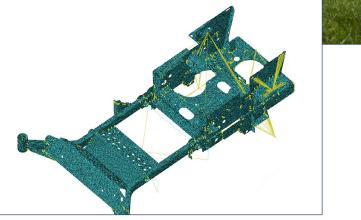
At the end of the redesign process, the new frame had 50 percent fewer parts (11 total) and cost less to manufacture than its predecessor. Testing time and costs were also reduced. When the new mower went through final field tests, Ariens engineers' confidence in their simulations was supported by the product's improved performance.
